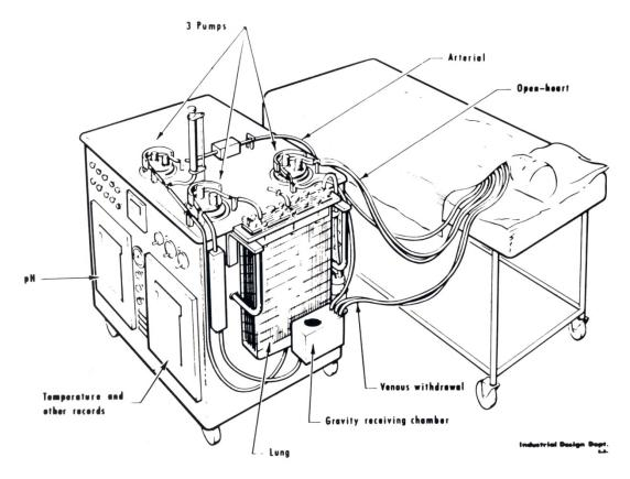
The IBM Heart-Lung Machine, or Oxygenator III
